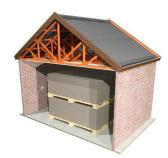
All Kalsi boards must be stored flat on pallets and placed inside covered and dry conditions, optimising protection for stored boards against exposure to weather and other unfavourable conditions.
